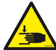
8. Crushing of hands hazard
