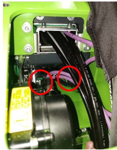
Figure 23. Telescope chain pulley wheel greasing points at the lower and upper boom linkage piece end
