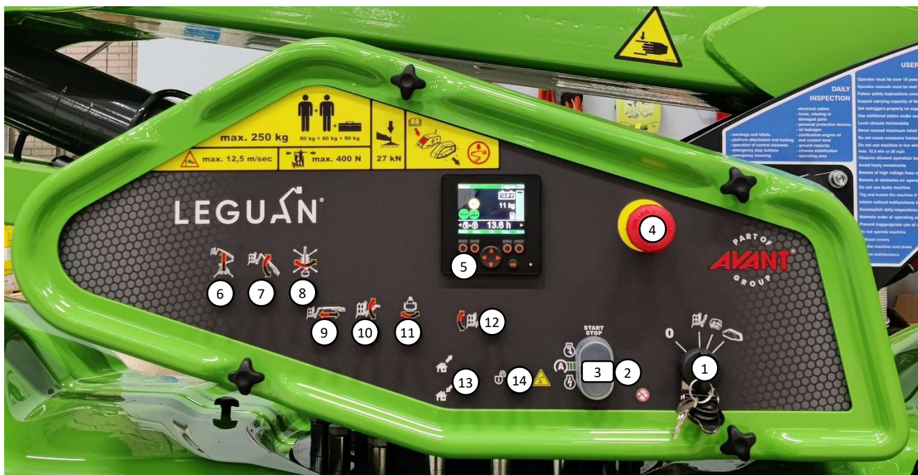
Figure 8. Lower control panel
